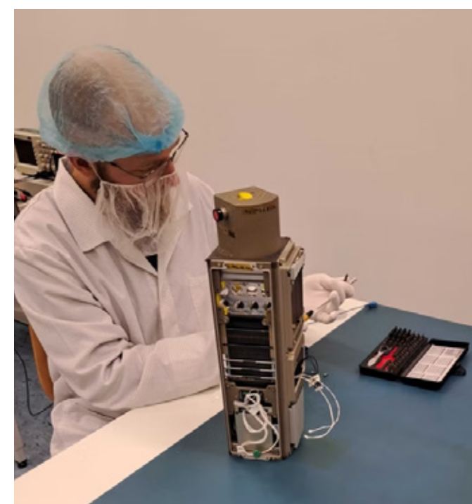
SPiN-2 platform integration at GOS Premises, Copyright: SPiN
